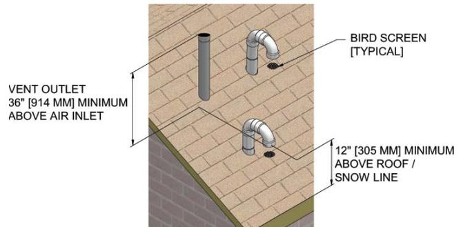
5. Locate terminations so they are not likely to be damaged by foreign objects, such as stones or balls, or subject to buildup of leaves or sediment.
