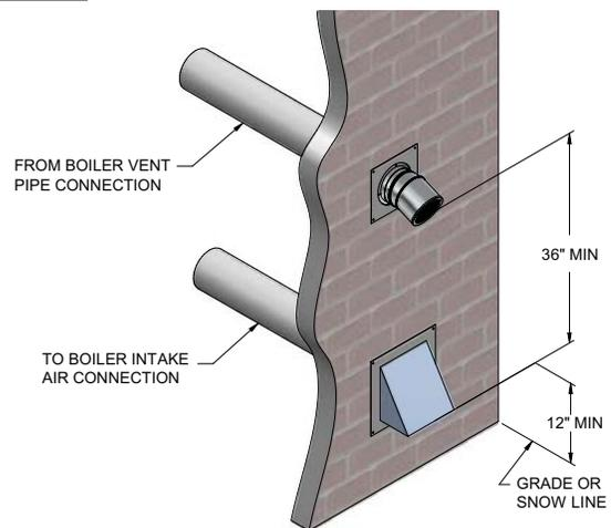
3. Maintain clearances as shown in FIG.'s 4-1 thru 4-3, pages 21 and 22. The vent termination should not be located in traffic areas such as walkways, adjacent buildings, operable windows, or doors. Also maintain the following:
