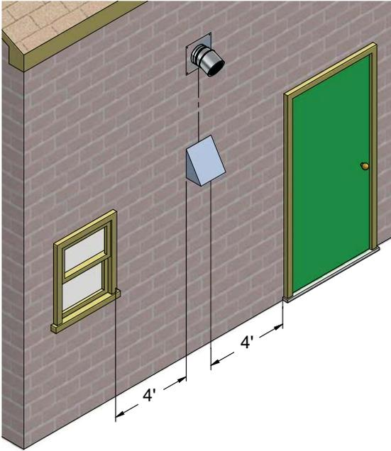
**Figure 4-3** Clearance to Forced Air Inlets
