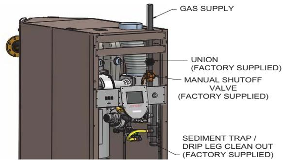
2. Support piping with hangers, not by the boiler or its accessories.
