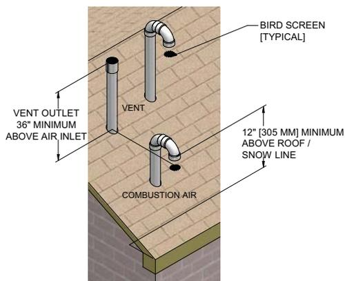
**Figure 3-2** Vertical Termination of Air and Vent w/Rain Cap
